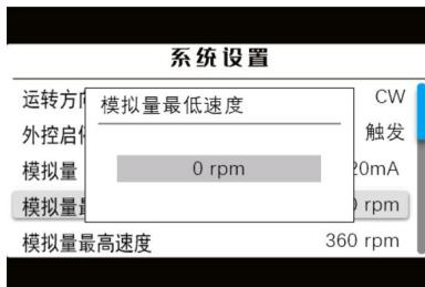
使用数字键盘输入模拟量最大值对应的转速，按
