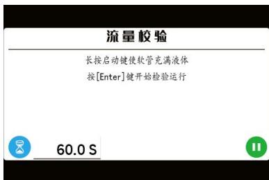
确保管子中已充满液体，长按
